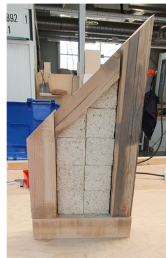
1/1 scale model of the construction system
